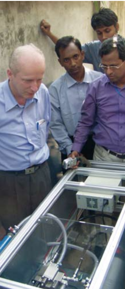
Figure 5. Field tests on arsenic removal in Bangladesh using a small scale desalinator.
