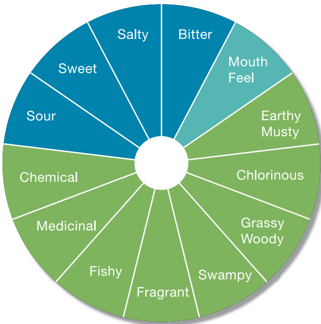
Figure 1. A taste and odour wheel. Adapted from Mallevalle and Suffet, 1987.
